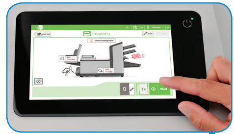
Full-color 7" touchscreen control panel with graphical interface and paper / envelope presence sensors
